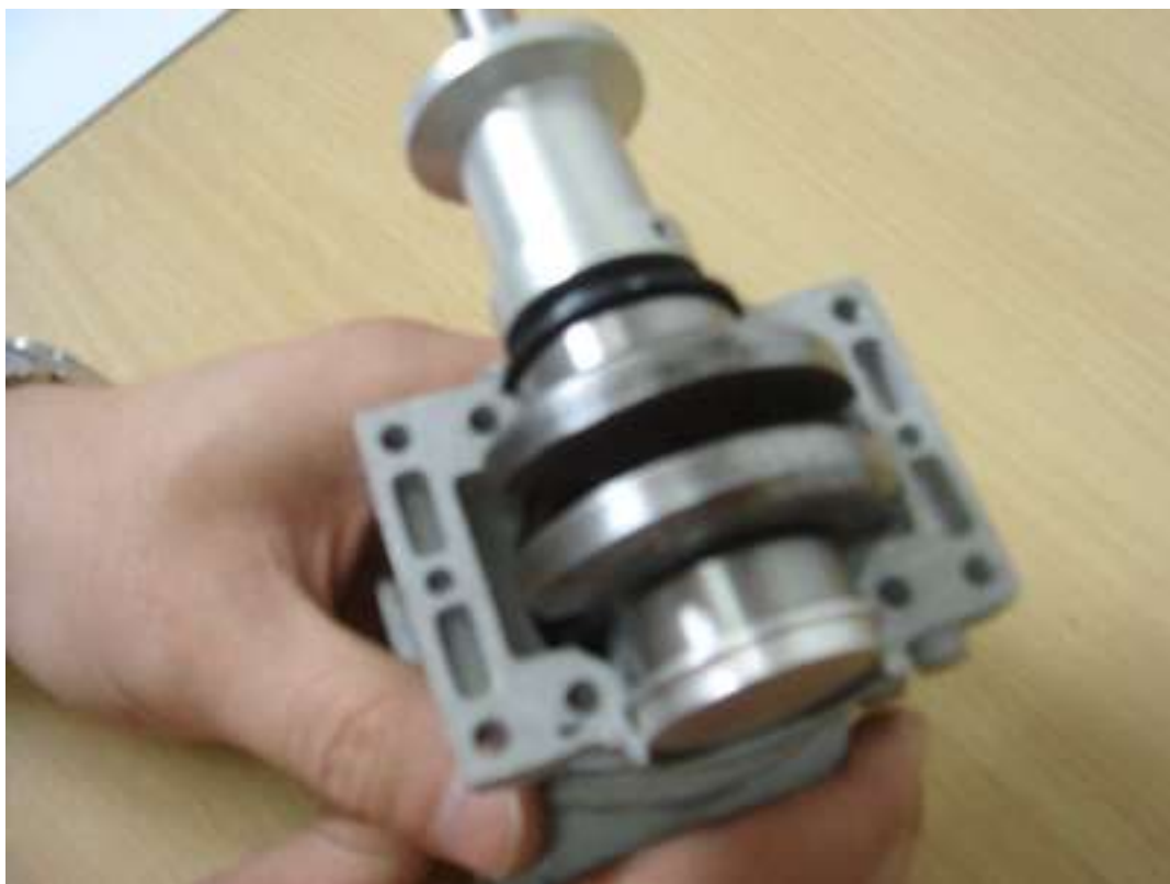
11: (Installation of the cylinder head with the crankshaft and piston assembly) (Parts required): (Crankcase bottom) 40120 x 1, M5X? (Screw) X4, M5 (lock washers ?)X4, (Sealant)
