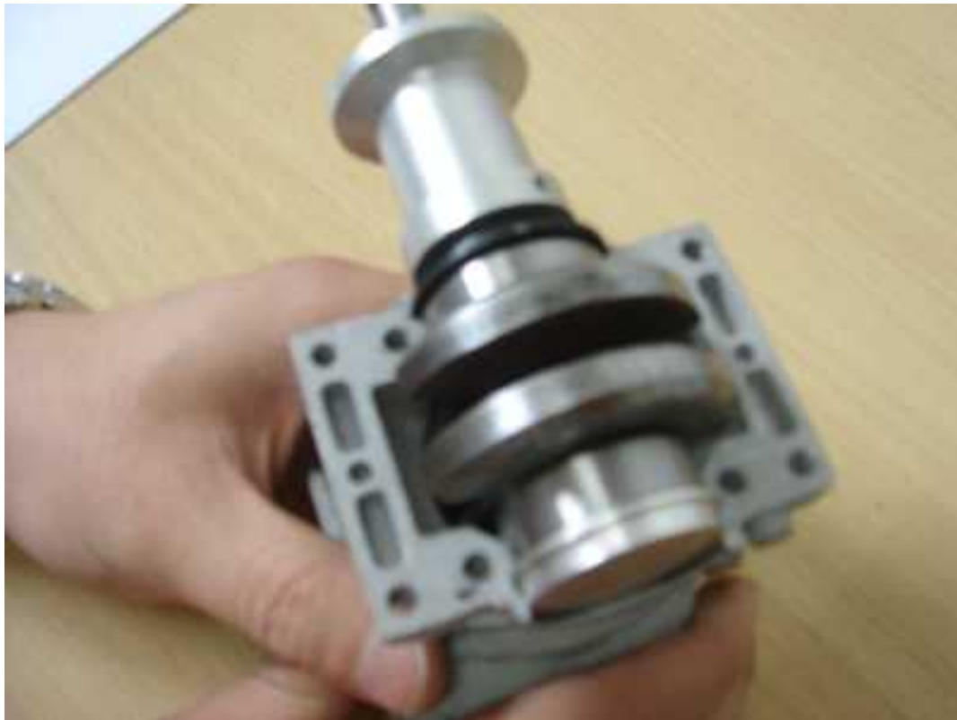
11. (Installion Zylinderkopf mit Kurbelwelle und Kolben) (Parts required) : (Crankcase bottom) 40120 x 1, M5X? (Screw) X4, M5 (lock washers ?)X4, (Sealant)
