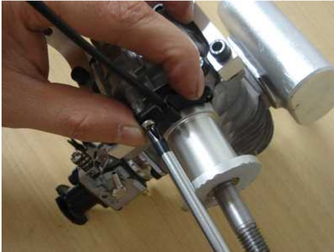
17, (Montage Entlüftungsschlauch) (Parts required) : Tubing 40250 x 1
