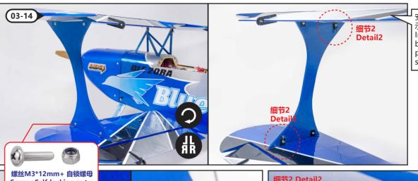
安装机翼支架,如图所 示,并注意几处细节。 Install the wing bracket as shown, and pay attention to several details.
