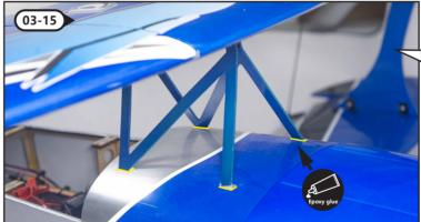
安装固定好左右机翼支架后,最后粘固中间支架。用环氧胶粘固, 粘合时保持上机翼平直。 After installing and fixing the left and right wing brackets, finally fix the middle bracket. Use epoxy adhesive to bond and keep the upper wing straight during bonding.
