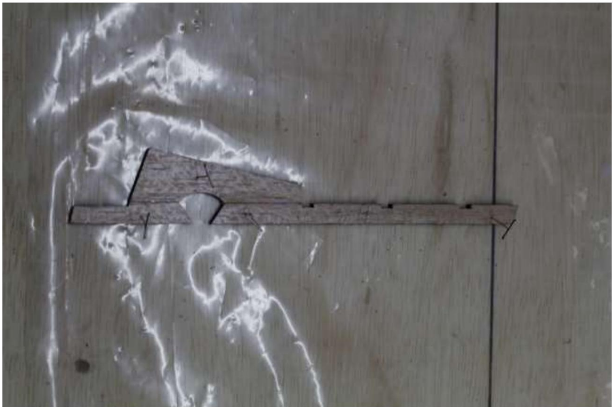
Staple and glue the front strip of the rudder flap (H16, H19) with connector (H15) onto the building base.
