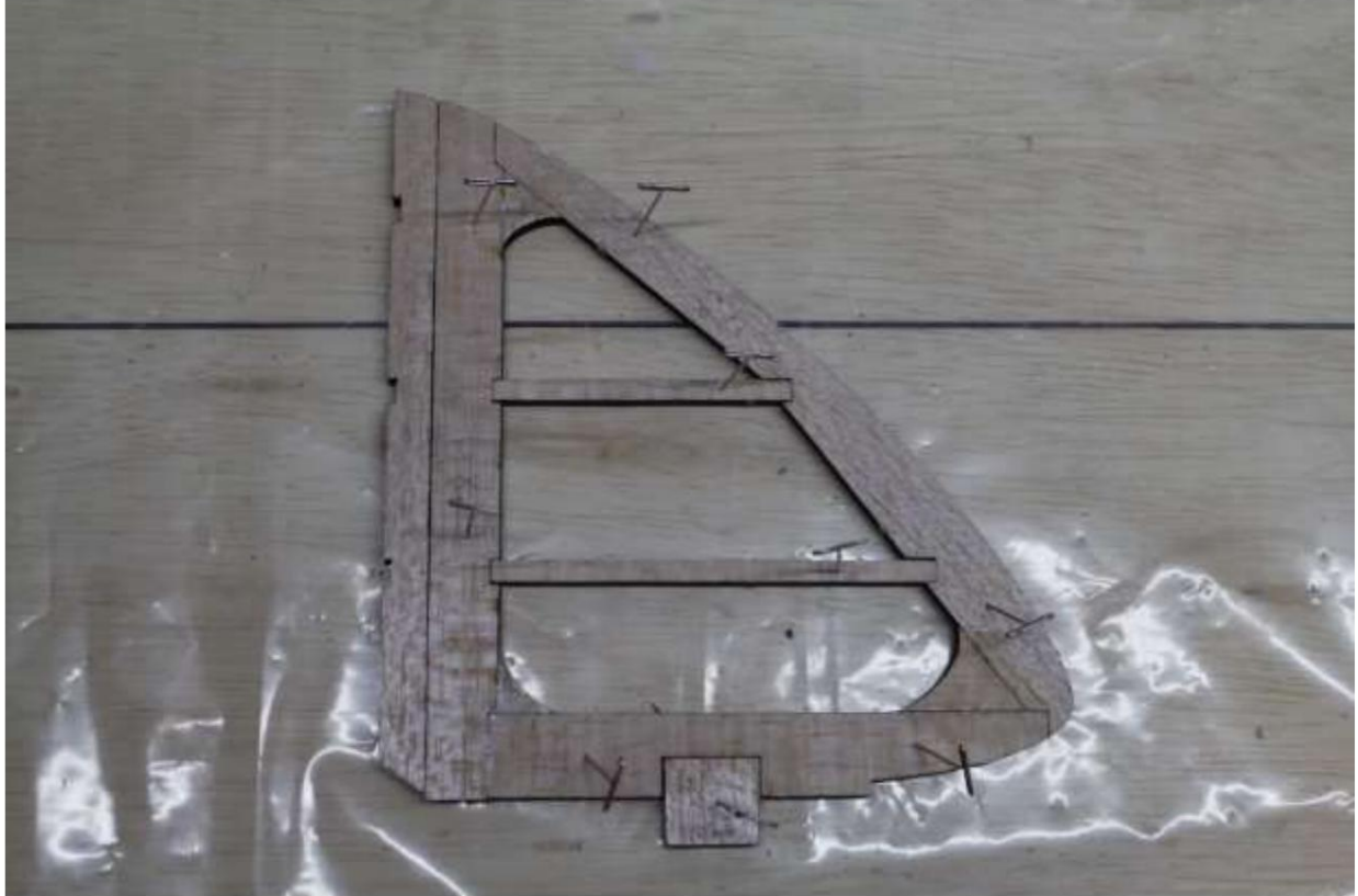
Glue in corner reinforcements (L10, H11).
