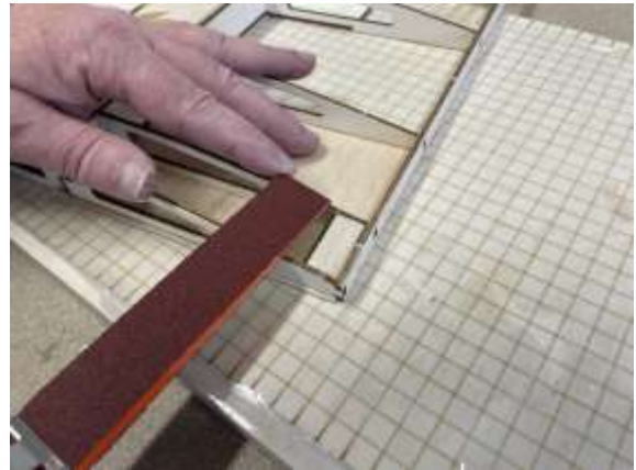
Now glue the upper planking made of 1.7mm balsa board. Sand any excess planking flush with the ribs.
