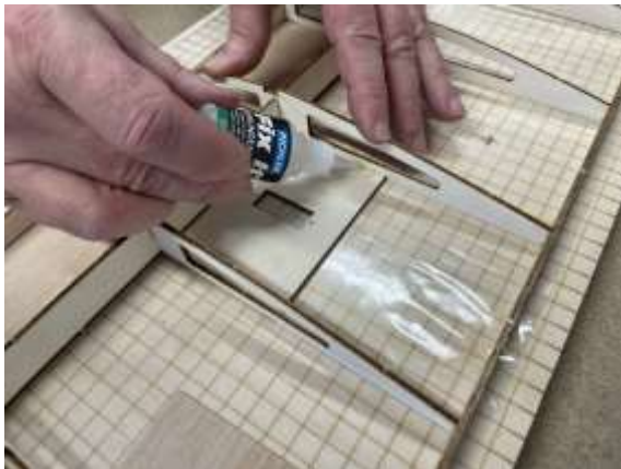
Glue in servo board D2.
