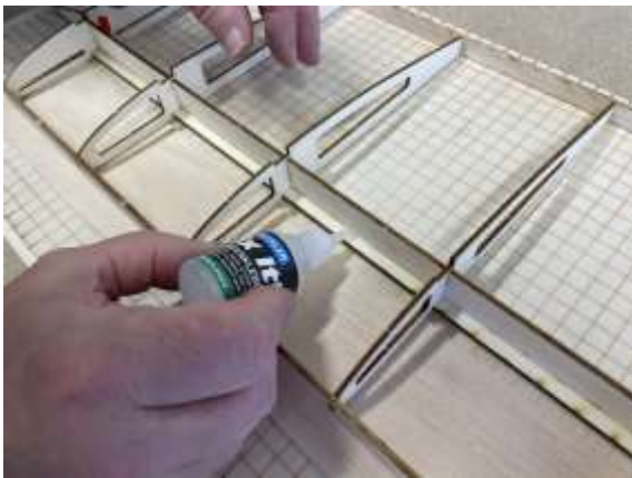
Glue in servo board D2.
