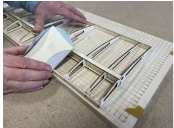
Sand strip G1 / G2 to match the ribs.
