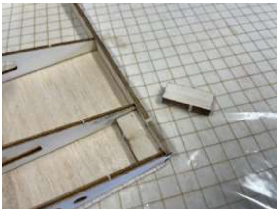
Glue in filler pieces H3 as shown as reinforcement.
