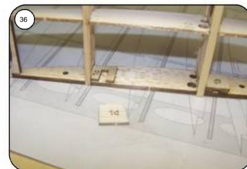
Glue pockets for the tensioning eyes 1a to 1d onto the inside of rib 1 according to the plan.
