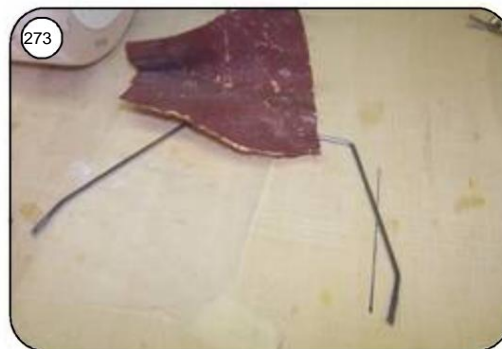
Sand the rear landing gear wire on all adhesive surfaces with sandpaper.
