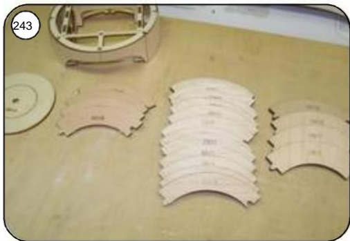
Parts for the front hood area Select Mh11, Mh12, Mh13 and Mh14.
