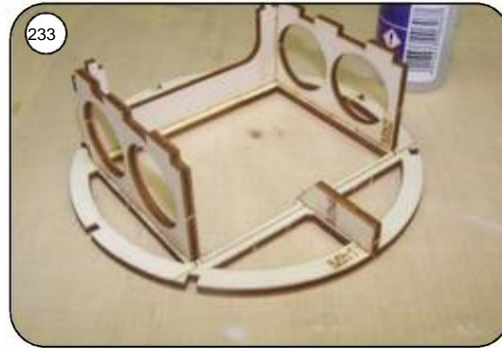
232 Glue the spacer frame made of Mh2 and Mh3 together into the front ring frame Mh1 Insert and glue with superglue.
