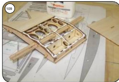
109 Glue the upper paneling Mo14 to the middle piece with white glue and up to Secure drying with needles.
