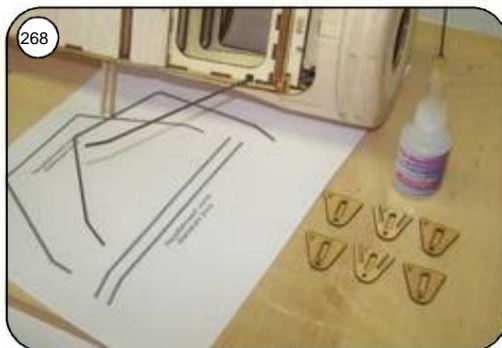
Produce wires for the chassis according to the bending instructions.
