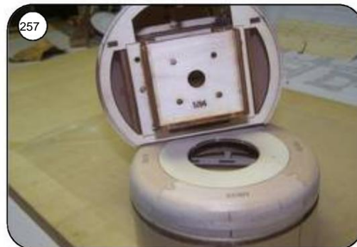
Temporarily attach the finished motor mount to the fuselage head with 2 screws Put on the engine hood and screw it to the engine support from the underside.
