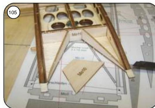
Fit half ribs Mo12 and glue them to Mo10 and Mo11 accordingly. Remove the rear bridge from Mo10.
