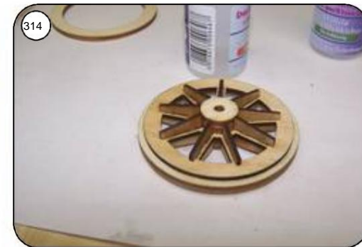
Glue in the doubling rings for the axle and reinsert the remaining spokes.
