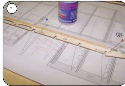
Place the cut-to-length spar strap on F1 and glue it together with a thin layer of superglue.
