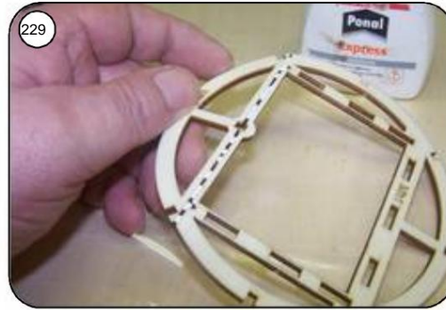
228 Glue the front ring frame for the bonnet Mh1 together with adhesive tape, fold it open and put white glue into the gap. Until Place weights to dry thoroughly.
