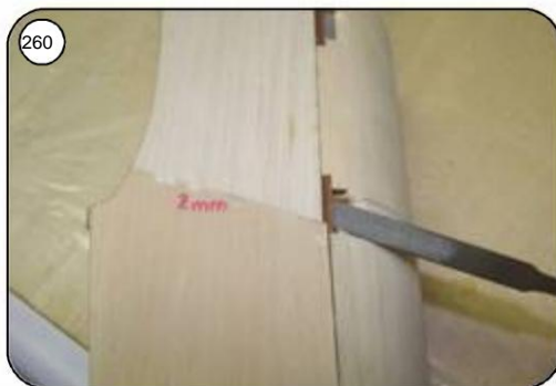
File pockets for the canopy struts with a flat key file and the Insert the canopy easily.
