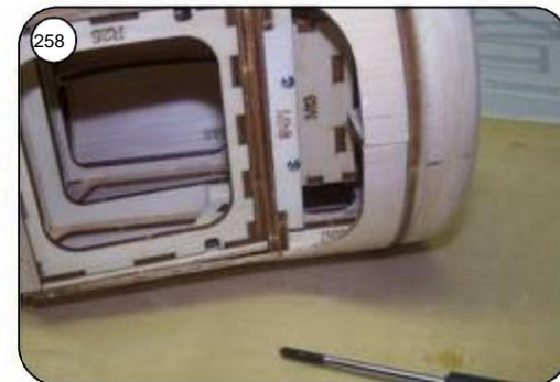
Temporarily attach the finished motor mount to the fuselage head with 2 screws Put on the engine hood and screw it to the engine support from the underside.
