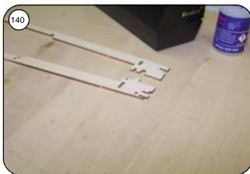
Staple the inner straps for the rear fuselage R6 and R7 together at the end of the fuselage with adhesive tape and glue it with superglue.
