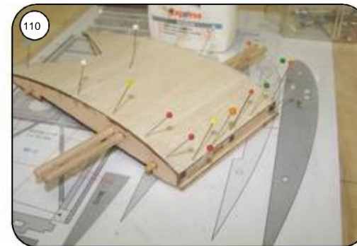
109 Glue the upper paneling Mo14 to the middle piece with white glue and up to Secure drying with needles.
