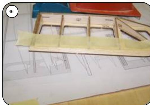
Sand the end strip according to the plan as for the wing.
