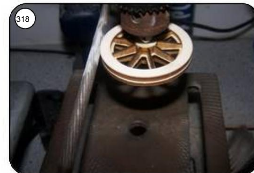
Screw a longer M4 threaded screw into the wheel axle. The bike with the Clamp the screw in a drill and at low speed with a Rub/turn the rim base with a round file.
