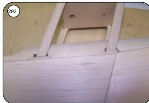
Fit the canopy into the fuselage again and the locking bridges in the fuselage. Fit in, pay attention to ease of movement here too.
