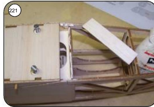
220 Fit the lower surface center piece into the fuselage, if necessary ream out the holes for the plug-in pegs a little. middle floor Insert and glue in the lower planking for the transition between the end strip and the fuselage.
