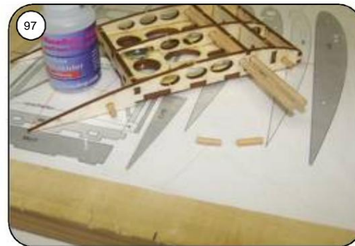
Cut the beech end cable to 3 x 15 mm and insert it Glue in the ribs Mo1.
