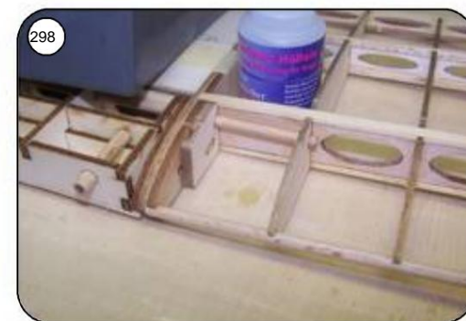
Put weight on the center of the surface and place supports on the right and left of rib 8 and put weight on the outer wing. Plug-in dowel (beech) with thin glue superglue to the comb spar and the ribs.
