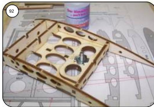
M4 impact nut with corresponding screw pull in and secure with superglue.
