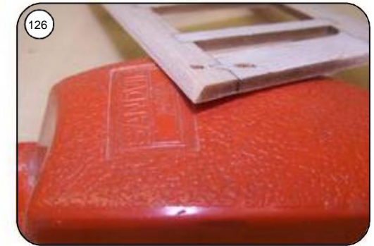
Hinge edge slanted towards the bottom Sand and round outer edges.
