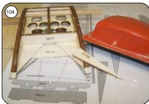
Fit half ribs Mo12 and glue them to Mo10 and Mo11 accordingly. Remove the rear bridge from Mo10.
