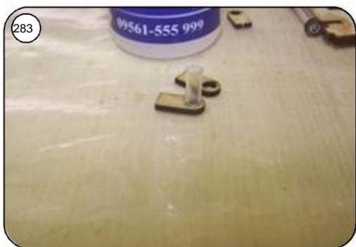
283 Glue the Bowden cable section into bearing R48, the distance is determined by the recesses on the underside of the fuselage, components in Glue the recesses on the underside of the fuselage, with the Bowden cable section protruding downwards.
