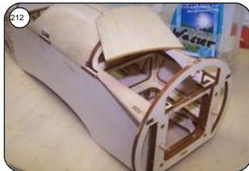
Also moisten the front paneling R46 from the outside with water and pre-bend it. Put the planking on and glue it on the inside with superglue.
