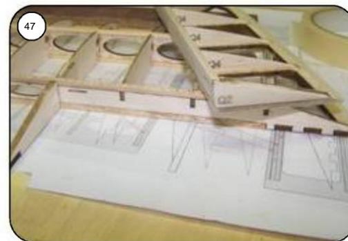
Sand the hinge edge for the desired hinge design, see plan for cuts.
