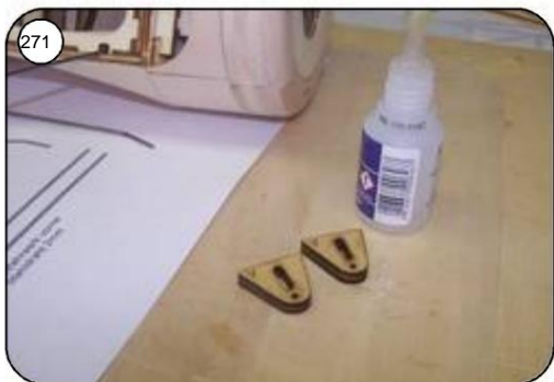
Suspension settings thoroughly all around soak/harden in thin superglue.
