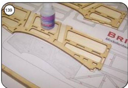
Glue from the inside with thin superglue (under the plywood let it creep in).
