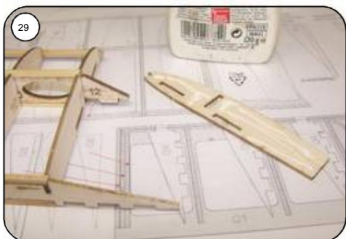
Coat rib 12 with white glue and push it onto the end of the surface, secure it additionally with a second.
