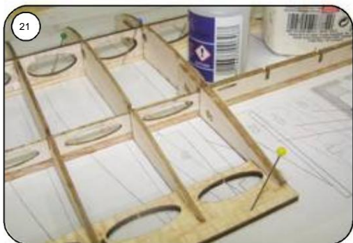
Glue in reinforcement rib 8c.
