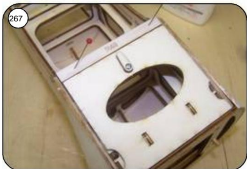
Fit the lid into the bottom of the fuselage and the planking strip R49 on the Glue on frames.
