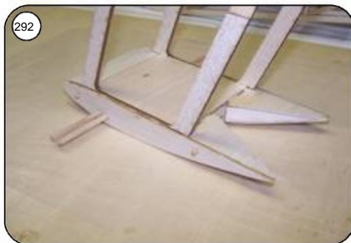
Round out and clean the doubling and struts in the area that will be visible later slur. Fit the canopy again into the middle of the area, making sure it moves easily. Cut the M4 plastic screw to length.
