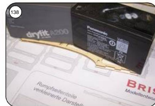
Glue the fuselage inner wall reinforcement R2 onto the fuselage side panel R1 in line with the contour, only including the larger adhesive areas Apply white glue, do not allow any glue to penetrate into the pockets in R2. Use weights until dry prove.
