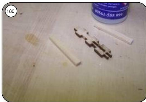
180 Double the frame R30 on both sides with remaining pieces of 4x2mm pine and then Drill out the bridge at the bottom end with 2mm (spur insertion)
