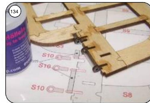
Lower hinge bearing (tube + Glue 2x S10) into the rudder. (Ruderhorn S11 after the Stretched)
