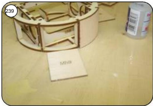
Paneling parts Mh9, starting from the top, 2 pieces each on the right and left. stick on. Bonding from the inside with thin superglue.
