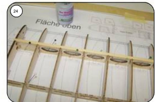
Cut the upper pine spar strap to lengths of 4 x 2 mm and stick it on with thick superglue.
