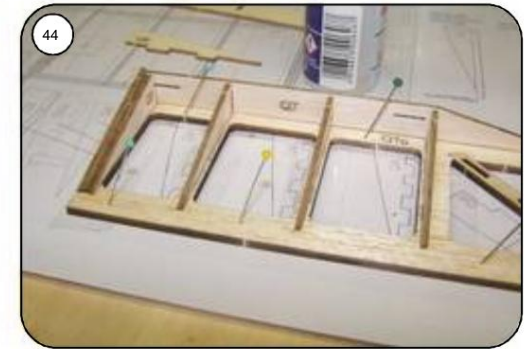
Push the doubling of the hinge strip Q7 onto the rib pins and glue it together. Glue in rib Q6.
