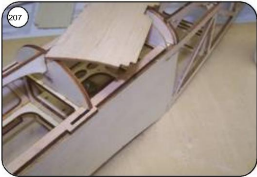
Hull back planking R45 on the Moisten the outside with water and carefully bend forward a little.
