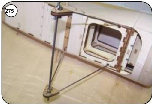
275 Mount the landing gear on the fuselage, front Chassis wires with 2K glue into the Glue in the suspension backdrops.
