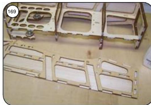
Opposite fuselage side part at the gluing points to the frame frame with glue Coat it and insert the frame frame, put weights on it again.
