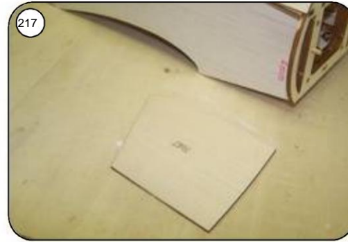
217 Moisten the planking again with water and bend forward.
