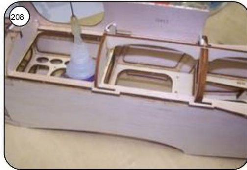
Place R45 on the fuselage side panel and with second from the inside Glue the frames together with white glue.
