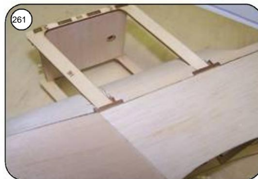
Temporarily attach the finished motor mount to the fuselage head with 2 screws Put on the engine hood and screw it to the engine support from the underside.
