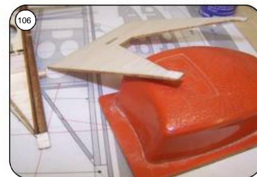
Upper planking Mo13 at the ends sand slightly at an angle (adhesive surface).
