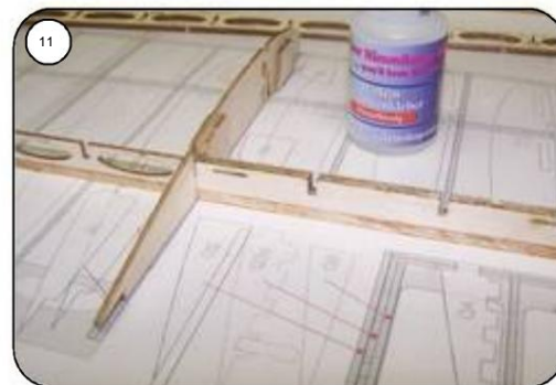
Insert rib 8 into the comb spar F1, align it according to the plan and carefully attach it.
