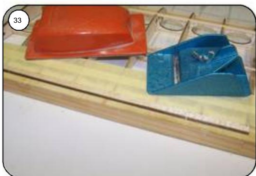
Sand the end strip at the end edge according to plan. Double-glued crepe strips glued to the ends of the ribs prevent them from being accidentally sanded.
