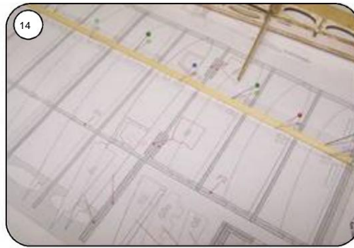
Tape the entire length of the underside of the spar strap with a strip of adhesive tape. Align the spar strap on the construction plan and fix it with pins using the adhesive tape.
