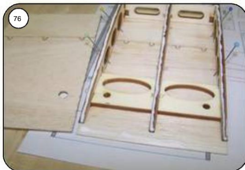
Sand the end edge of Mu13 diagonally (adhesive edge), glue the planking onto the rib framework with white glue and use needles to back up.
