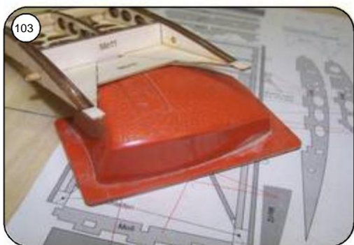
Ends of planking Mo10 light Sand diagonally (adhesive surface).
