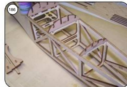
185 Align half frames R31, R31a and R32 on the corresponding frames and glue them on
