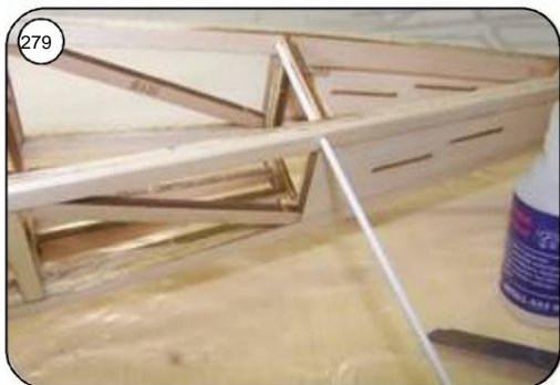
279 Front and rear connecting tubes (Bowden cable 2mm) for the tail unit strut into the corresponding holes in the Glue the fuselage in place and cut it off flush with the outside of the fuselage.
