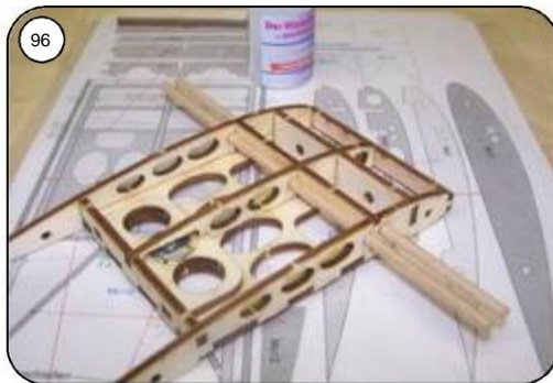
Cut round beech rods 4 x 170 mm and glue them into the middle of the middle piece.
