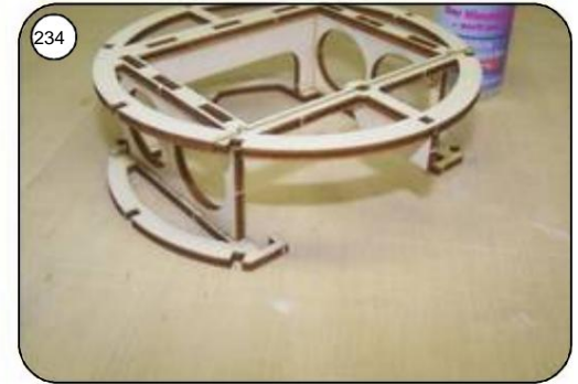
234 Insert the finished assembly into the rear ring frame Mh5 and also Glue superglue.
