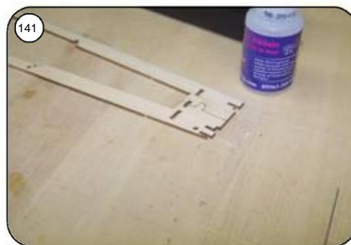
Staple the inner straps for the rear fuselage R6 and R7 together at the end of the fuselage with adhesive tape and glue it with superglue.
