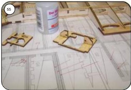
Release the parts for the servo mount from the laser board and glue the servo mount together and insert it into the surface as a test.
