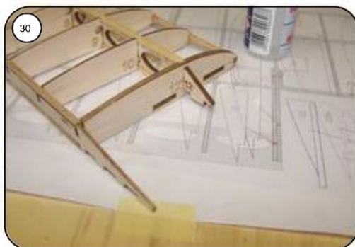
Coat rib 12 with white glue and push it onto the end of the surface, secure it additionally with a second.
