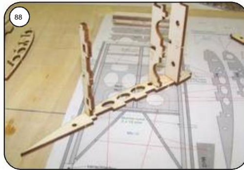
Webs Mo2, Mo3 and Mo5 in rib Mo1 Glue in at right angles.
