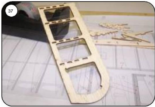
Cover the slots on the underside of the aileron base Q1o with adhesive tape.
