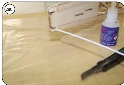
279 Front and rear connecting tubes (Bowden cable 2mm) for the tail unit strut into the corresponding holes in the Glue the fuselage in place and cut it off flush with the outside of the fuselage.
