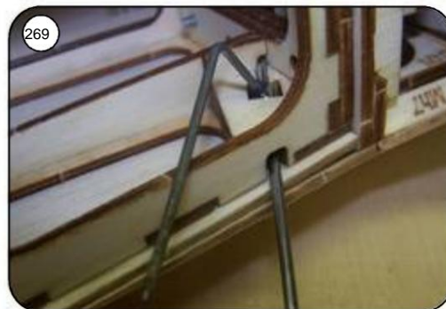
Front landing gear wires into the mounts Insert into the fuselage and with a 2mm adjusting ring to back up.
