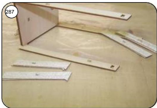
Glue the extensions for the canopy struts B7 to B10 to the inside and outside of the struts. Fill the transition between doubling and planking.
