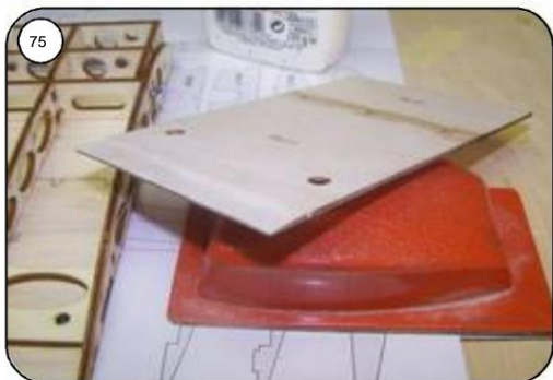
Sand the end edge of Mu13 diagonally (adhesive edge), glue the planking onto the rib framework with white glue and use needles to back up.
