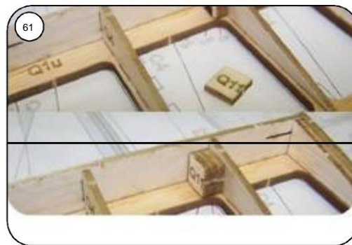
In addition, the pocket for the rudder horn is made from parts Q9, Q10 and Q11 glued in.
