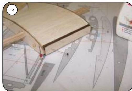
113 Fit the nose strip Mo16 and glue it on. Sand the entire middle section cleanly.
