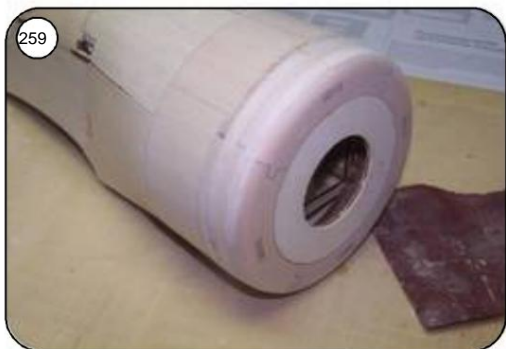
The shape of the hood can now be sanded to match the fuselage head become.
