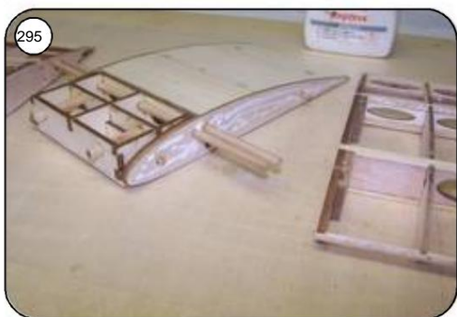
Halves of the area with the respective middle piece on the connecting ribs are coated with white glue. Glue together and clamp together with tape strips.
