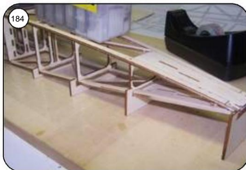
183 Put weight on the front area of the fuselage (flat on the building board) then the Assemble supports St1 to St4 in the rear area according to the plan and the rear of the fuselage pull together, weight on top. Bonding with thin superglue.
