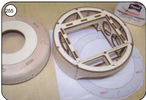
Glue the finished nose block to the rear part of the hood with white glue.
