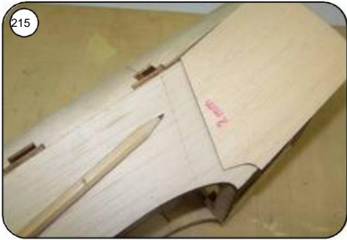
215 Place planking R47 (transition between fuselage and ring frame) and the end edge on the fuselage mark. Grind the end edge of the planking diagonally as a support on the hull.
