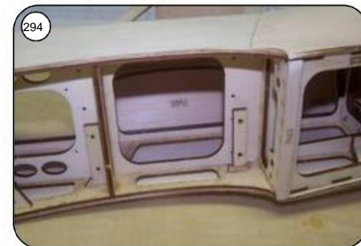
Fit the canopy into the fuselage again and the locking bridges in the fuselage. Fit in, pay attention to ease of movement here too.
