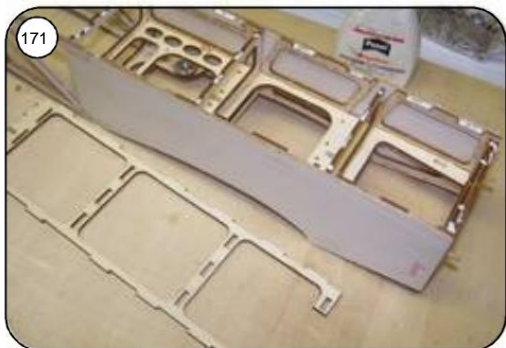
Glue the upper fuselage cover with white glue and secure it with superglue if necessary.
