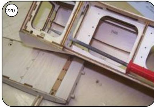
220 Fit the lower surface center piece into the fuselage, if necessary ream out the holes for the plug-in pegs a little. middle floor Insert and glue in the lower planking for the transition between the end strip and the fuselage.
