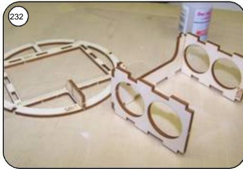
232 Glue the spacer frame made of Mh2 and Mh3 together into the front ring frame Mh1 Insert and glue with superglue.
