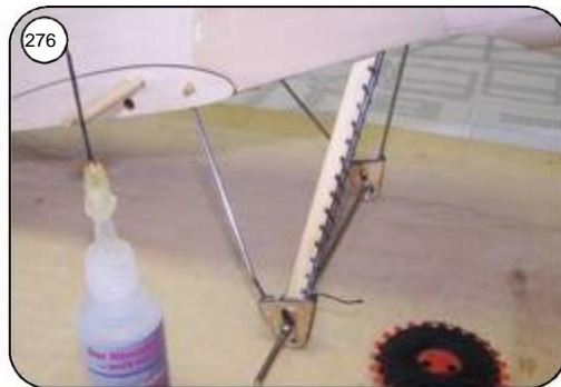
276 Sew the undercarriage panels to the undercarriage wires using household twine Glue with thin superglue. Chassis fairings to the suspension backdrops Glue with 2K glue.
