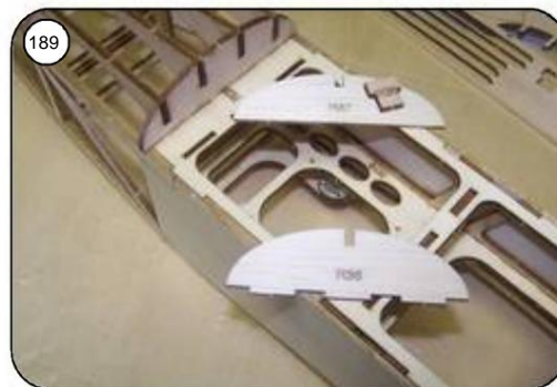
189 Glue half frames R36 and R37 together with the spacer R38, Planking support for the rear cockpit area.
