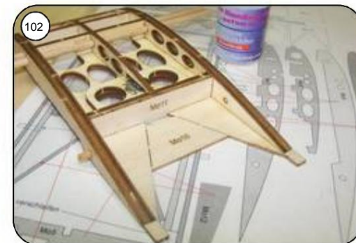
Glue the bottom end paneling made of Mo10 and Mo11 together into the middle section insert and glue.
