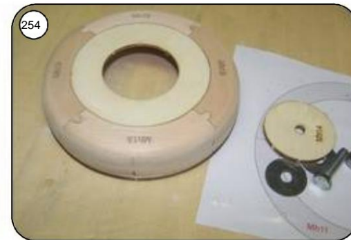
Nose block carefully at low speed _____ Grind/turn into shape, using the Do not sand the rear ring as this will later be attached to the rear part of the hood adjusted. Remove threaded screw and center piece from Mh14.
