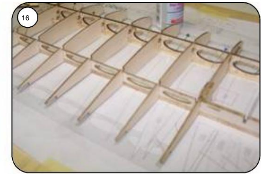
Insert ribs 2 to 7 and glue them in with Seku, while also gluing the comb spar F 3 to the spar belt.
