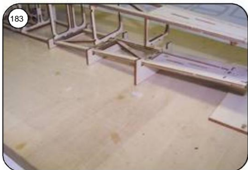
183 Put weight on the front area of the fuselage (flat on the building board) then the Assemble supports St1 to St4 in the rear area according to the plan and the rear of the fuselage pull together, weight on top. Bonding with thin superglue.
