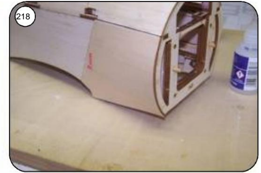
218 At the end edge with thick superglue, the rest from the inside Glue with thin superglue.
