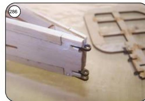
286 Upper bearing R48 in the fuselage cutout align and glue.
