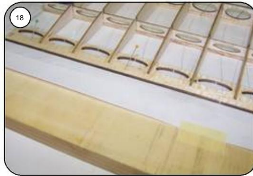
Push in the end strip F4, secure it with pins and glue it to the ribs
