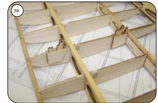
Put the bracing and struts into the appropriate pockets as a test. Insert, adjust if necessary. Final assembly only takes place after the covering.
