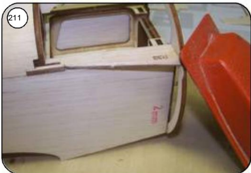
Planking support R39 slanted according to the curve of the ring frame grind.
