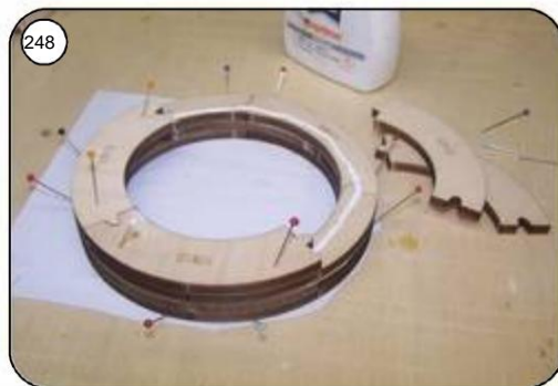
Next, a ring made of 4 parts Stick on Mh12 (turn again approx. 45°).
