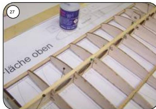
Cut the beech nose strip to around 4 mm and glue it in place.
