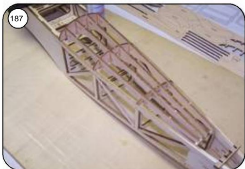
187 Carefully insert fuselage skirt strips R34 and R35 into the half frames and with these glue. Push in the end R33 and align it centrally on the fuselage. With Glue superglue.
