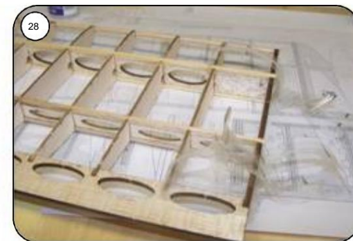
Remove the surface from the building board and remove the tape strips.
