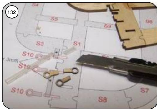
Cut the 3mm Bowden cable tube for the SR hinge according to the construction plan.
