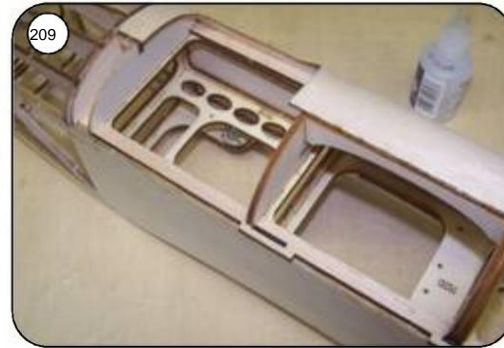
Bend the planking around the frames and along the upper middle bars Glue superglue. Apply opposite planking.
