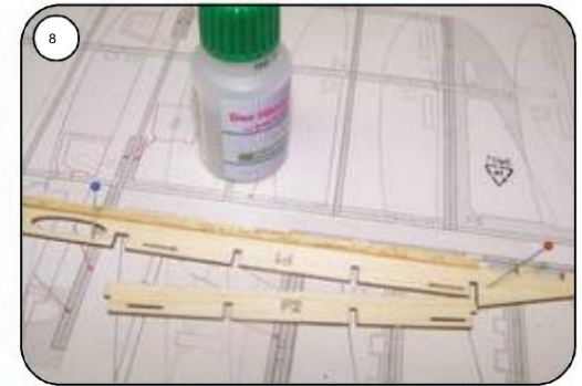
Glue reinforcement F2 to fit F1.
