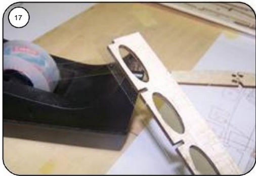
Tape the end strip F4 on the underside with adhesive tape (rib pockets).
