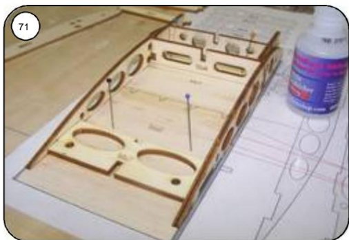
Assembly Mu3 - Mu6 (rib frame) together with the screw support Mu7 Glue onto the paneling Mu1 / Mu2.
