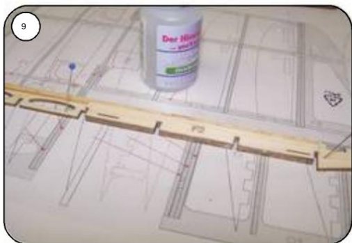
When gluing F2, pay attention to the position of the hinge slots.
