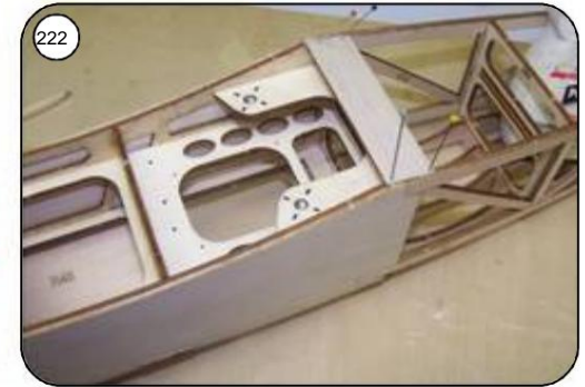
218 At the end edge with thick superglue, the rest from the inside Glue with thin superglue.
