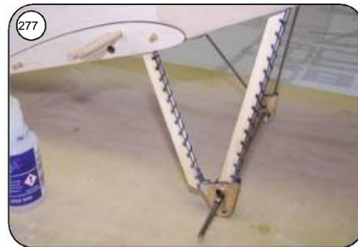
276 Sew the undercarriage panels to the undercarriage wires using household twine Glue with thin superglue. Chassis fairings to the suspension backdrops Glue with 2K glue.
