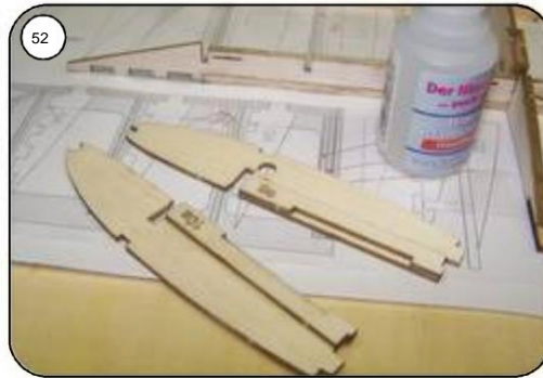
Glue the supports for the servo mount 9a and 10a onto the corresponding ribs 9 and 10 according to the plan, insert the ribs into the surface. Pockets for the tensioning eyes u1a to u1c. Glue u1d onto rib 1 according to plan.
