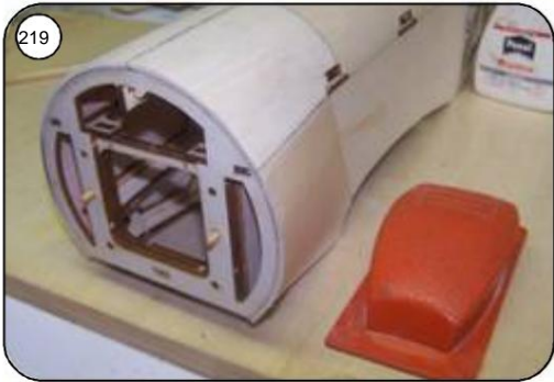
219 Excess planking on the hull head sand smoothly.
