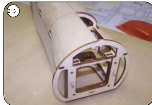
Also moisten the front paneling R46 from the outside with water and pre-bend it. Put the planking on and glue it on the inside with superglue.
