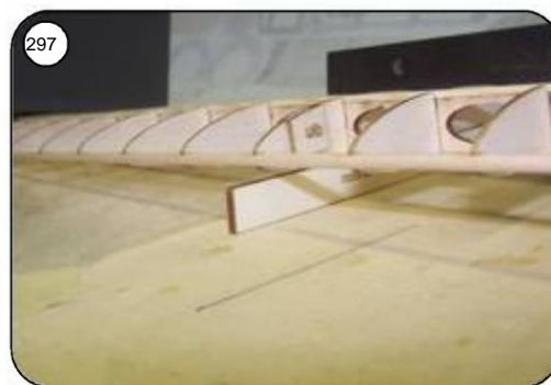
Put weight on the center of the surface and place supports on the right and left of rib 8 and put weight on the outer wing. Plug-in dowel (beech) with thin glue superglue to the comb spar and the ribs.
