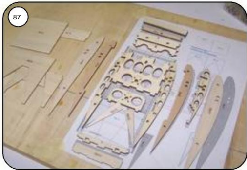
Components for the upper surface centerpiece from the laser boards and pre-sort.
