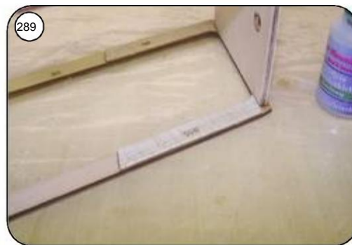
Glue the extensions for the canopy struts B7 to B10 to the inside and outside of the struts. Fill the transition between doubling and planking.
