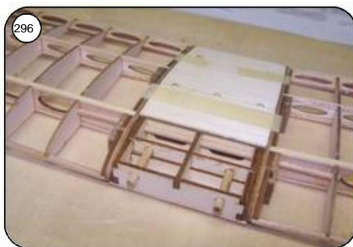
Halves of the area with the respective middle piece on the connecting ribs are coated with white glue. Glue together and clamp together with tape strips.
