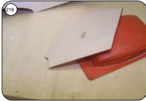
215 Place planking R47 (transition between fuselage and ring frame) and the end edge on the fuselage mark. Grind the end edge of the planking diagonally as a support on the hull.
