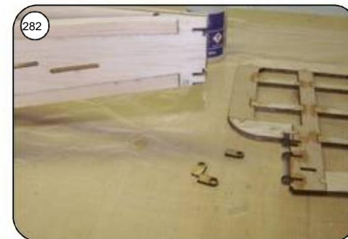
282 Select hinge bearing R48 and Bowden cable tube 3mm to approximately 8 mm LÇnge ablÇngen.
