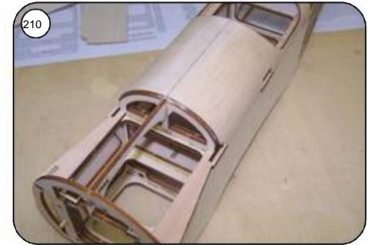
Glue the front ring frame R43 to the fuselage head and secure it with clamps up to Ensure drying.
