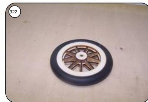
Put it on the rim as a test, final bonding only after Stretched der Felge.
