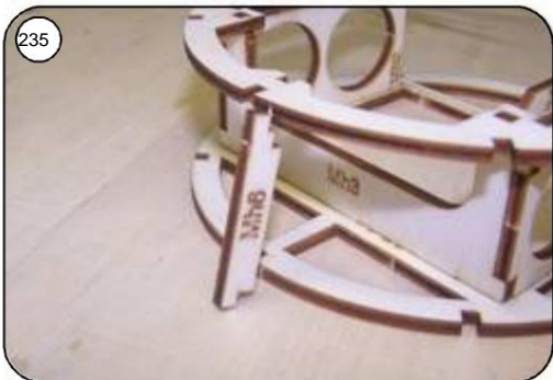
235 Connecting bridge Mh6 Get the ring bond Glue into the top of the hood frame. Double notch towards Mh5!!!
