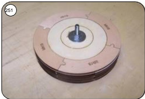
M6 threaded screw with suitable washers into the front panel Mh14 screw it in and clamp it in a drill.
