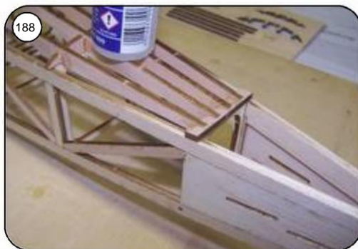
187 Carefully insert fuselage skirt strips R34 and R35 into the half frames and with these glue. Push in the end R33 and align it centrally on the fuselage. With Glue superglue.
