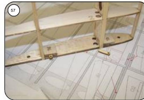
Put the bracing and struts into the appropriate pockets as a test. Insert, adjust if necessary. Final assembly only takes place after the covering.
