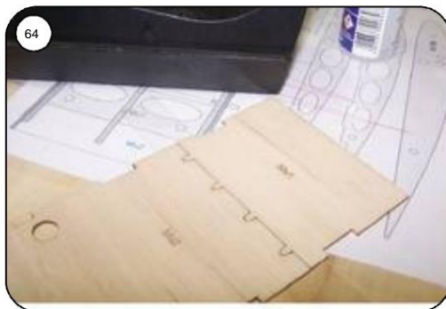
Paneling parts Mu1 and Mu2 on the Glue the later visible side together with adhesive tape and glue from the opposite side.
