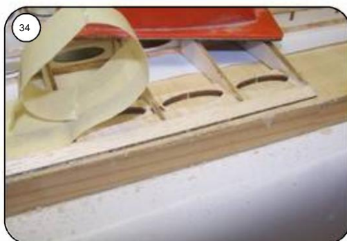
Sand the end strip at the end edge according to plan. Double-glued crepe strips glued to the ends of the ribs prevent them from being accidentally sanded.
