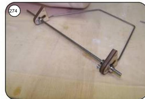
Suspension links with 3 mm adjusting rings Align and fix on the main axis Glue in the chassis wire with 2K adhesive.
