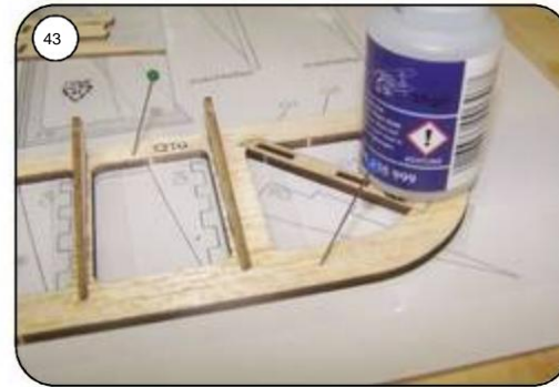
Fit the diagonal bar Q1a into the pocket of Q1 and glue it in place with superglue.
