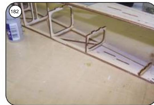
182 Insert frames R27 to R30 into the fuselage side part and use a dropper Attach superglue.
