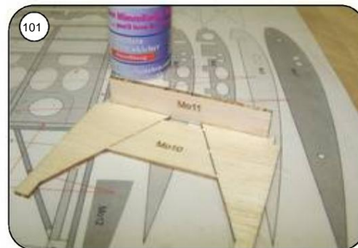
Glue the bottom end paneling made of Mo10 and Mo11 together into the middle section insert and glue.
