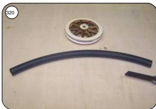
Foam rubber cord on 210 mm with a Cut the cutter knife and moisten it Cutter blade makes cutting easier.
