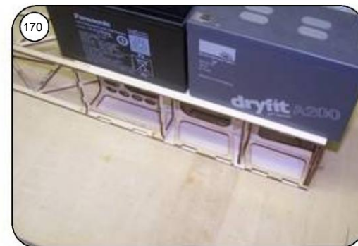
Opposite fuselage side part at the gluing points to the frame frame with glue Coat it and insert the frame frame, put weights on it again.
