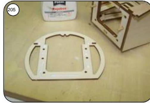
Glue the front ring frame R43 to the fuselage head and secure it with clamps up to Ensure drying.
