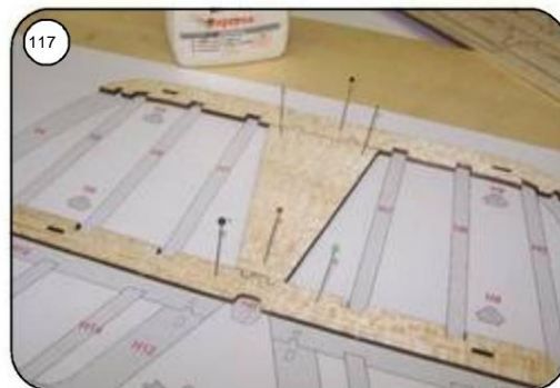
116 Align the center piece H2 and the nose strip H3 according to the plan and glue them together with white glue.
