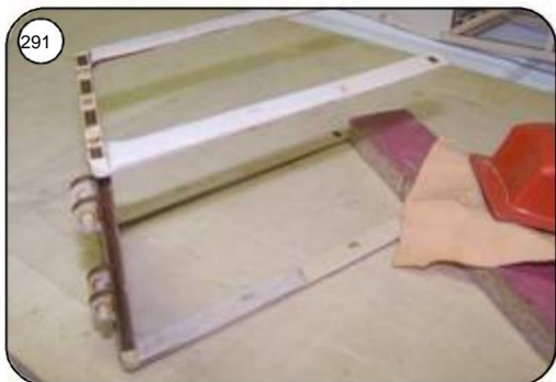
Round out and clean the doubling and struts in the area that will be visible later slur. Fit the canopy again into the middle of the area, making sure it moves easily. Cut the M4 plastic screw to length.
