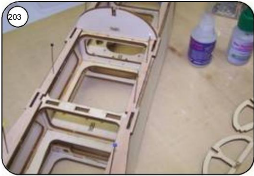
Glue in half frames R40, R41 and R42 together with the support strips R39, then stick on the bar R44.
