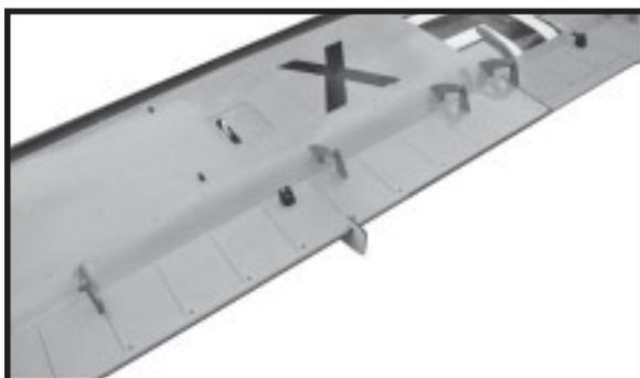
**INSTALLING THE FLAP LINKAGES.**
