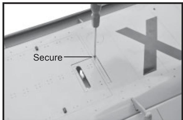
**INSTALLING THE FLAP CONTROL HORN.**
