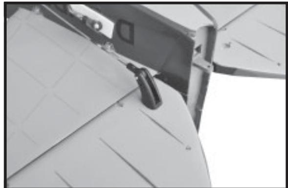
**Plastic parts of elevator pushrod.**
