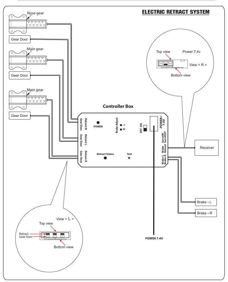
Note: Very important - DC volt input MUST BE 7.4v. If not, your system can be BROKEN.
