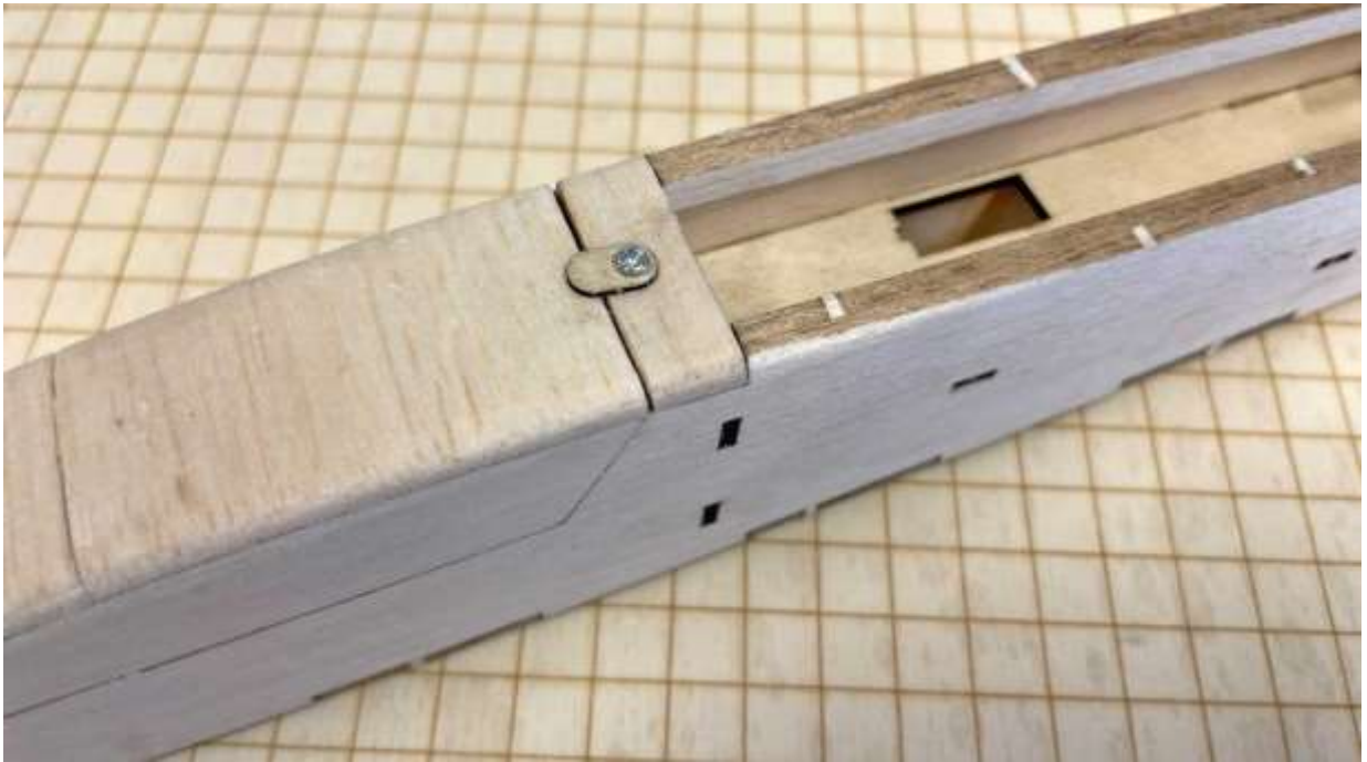
The G1 cabin bolt is fixed with a screw.
